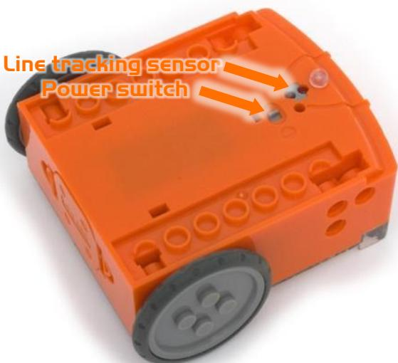
Edison's power switch and line tracking sensor
